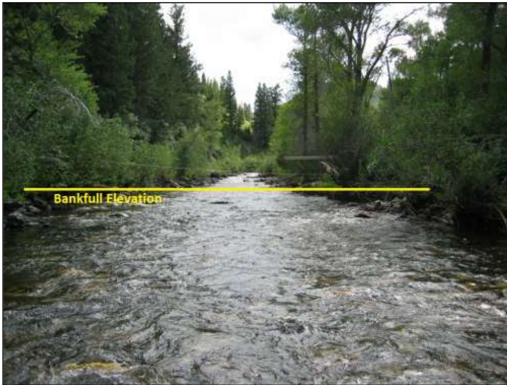
Figure 8 – Bankfull elevation associated with a break in slope or bankfull bench, intermittent scour lines and the base of alder ( Alnus sp.).
