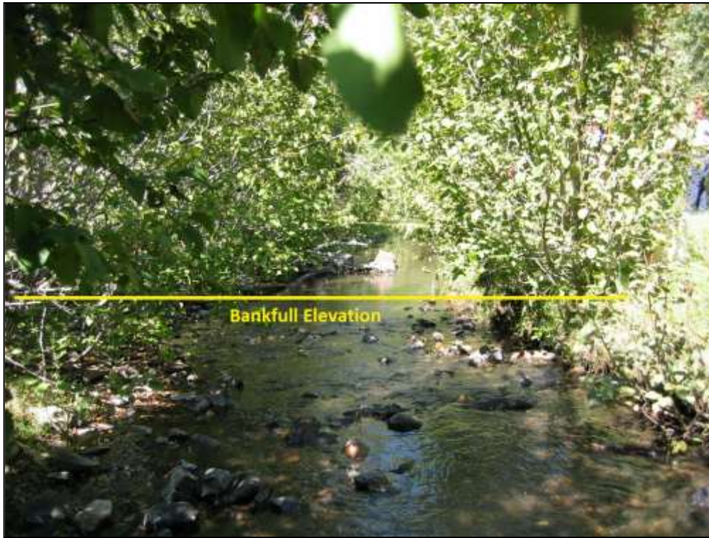
Figure 7 – Bankfull elevation associated with a break in slope or bankfull bench and the base of alder ( Alnus sp.).
