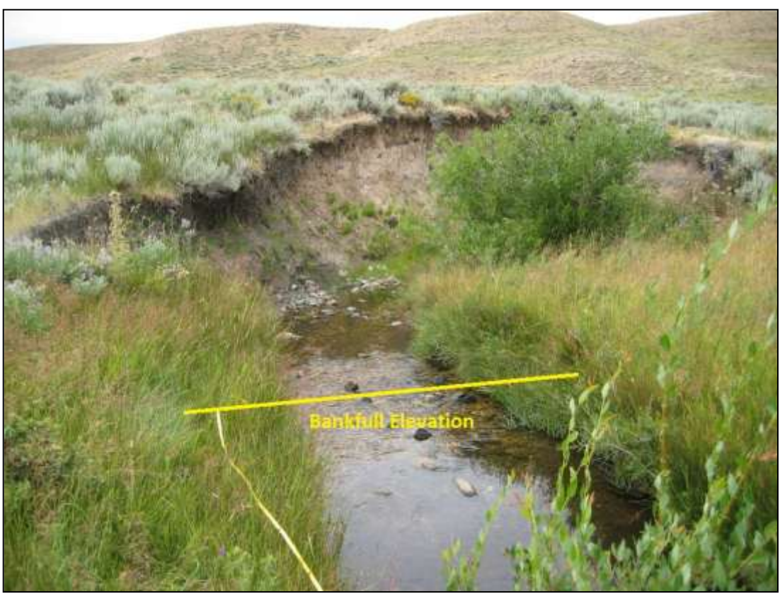
Figure 4 – Bankfull elevation associated with a break in slope, top of a point bar, a subtle floodplain, intermittent scour lines and the base of redtop ( Deschampsia sp.).
