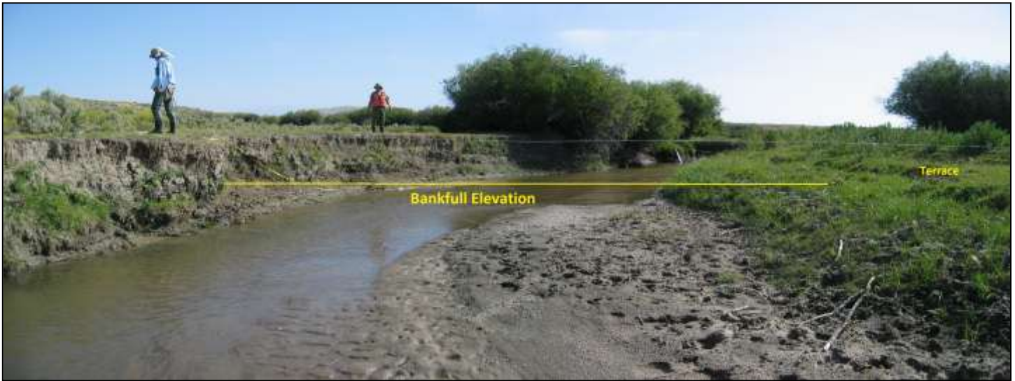
Figure 5 – Bankfull elevation associated with the top of a point bar and a break in slope at the bottom of a vertical bank with a scour line.
