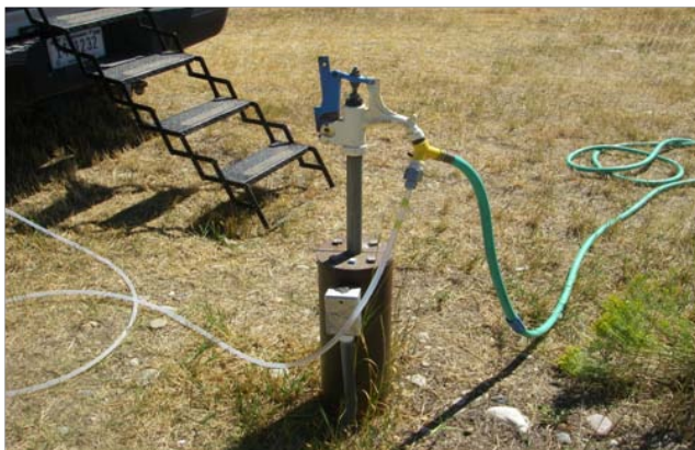
Figure 3 – Wellhead connections for groundwater sampling that lead to the mobile water-quality lab or a lawn sprinkler
